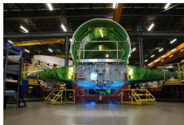
Set Dihedral, Sweep & Incidence Wing to Center Fuse Join
